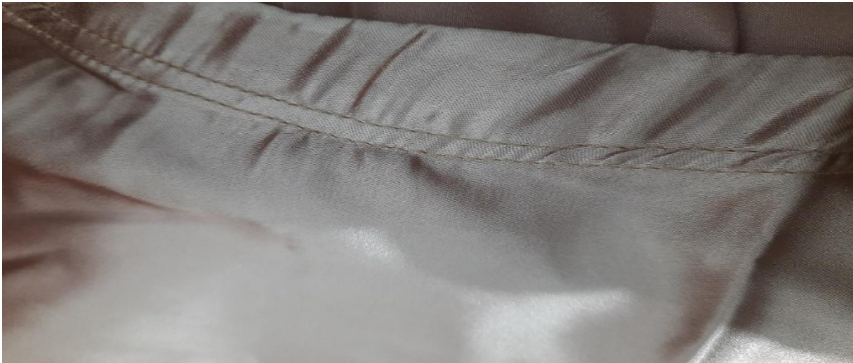
Figure: 2.3.3 Seam Puckering
