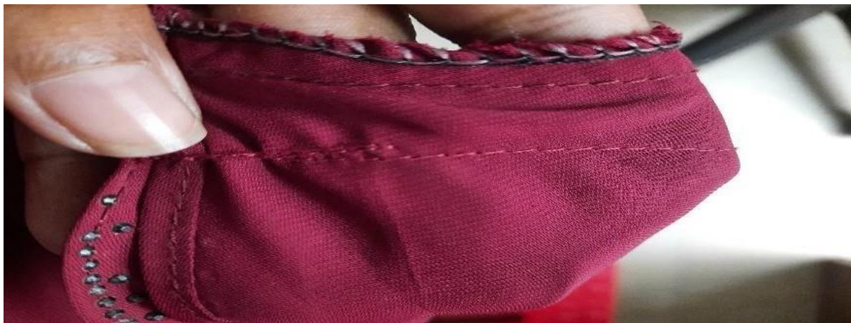
Figure:2.3.7 Variable Stitch Density
