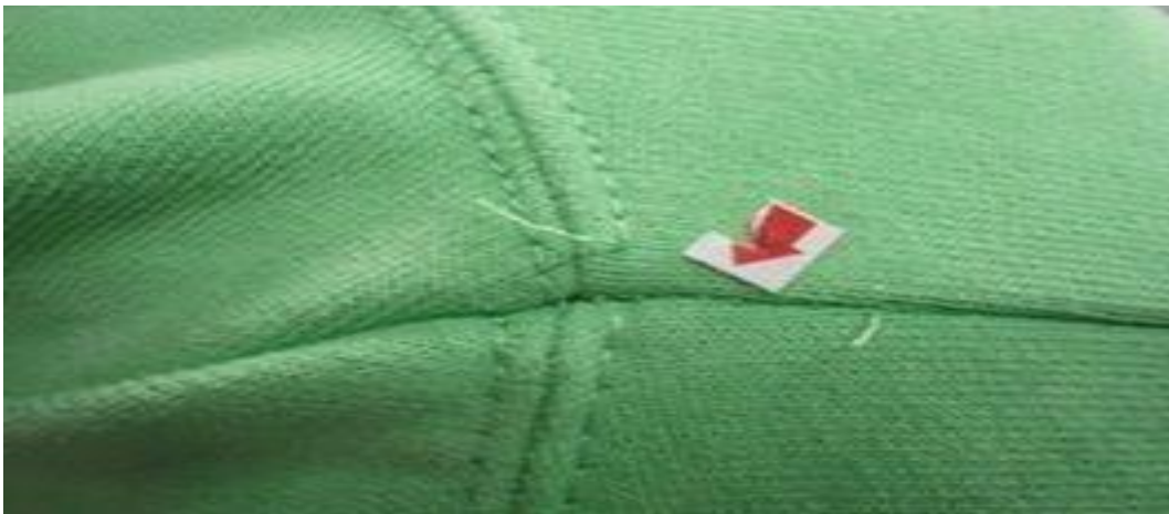
Figure: 2.3.4 Broken Stitch
