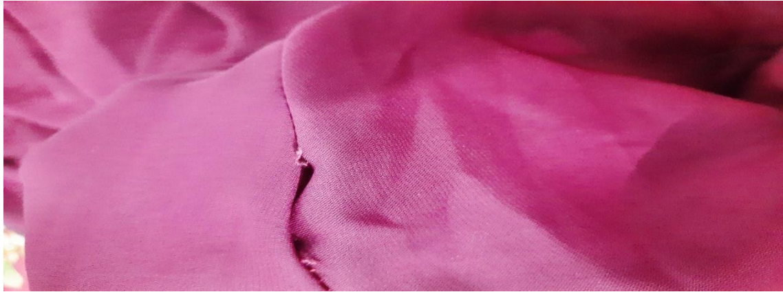
Figure: 2.3.6 Open Seam
