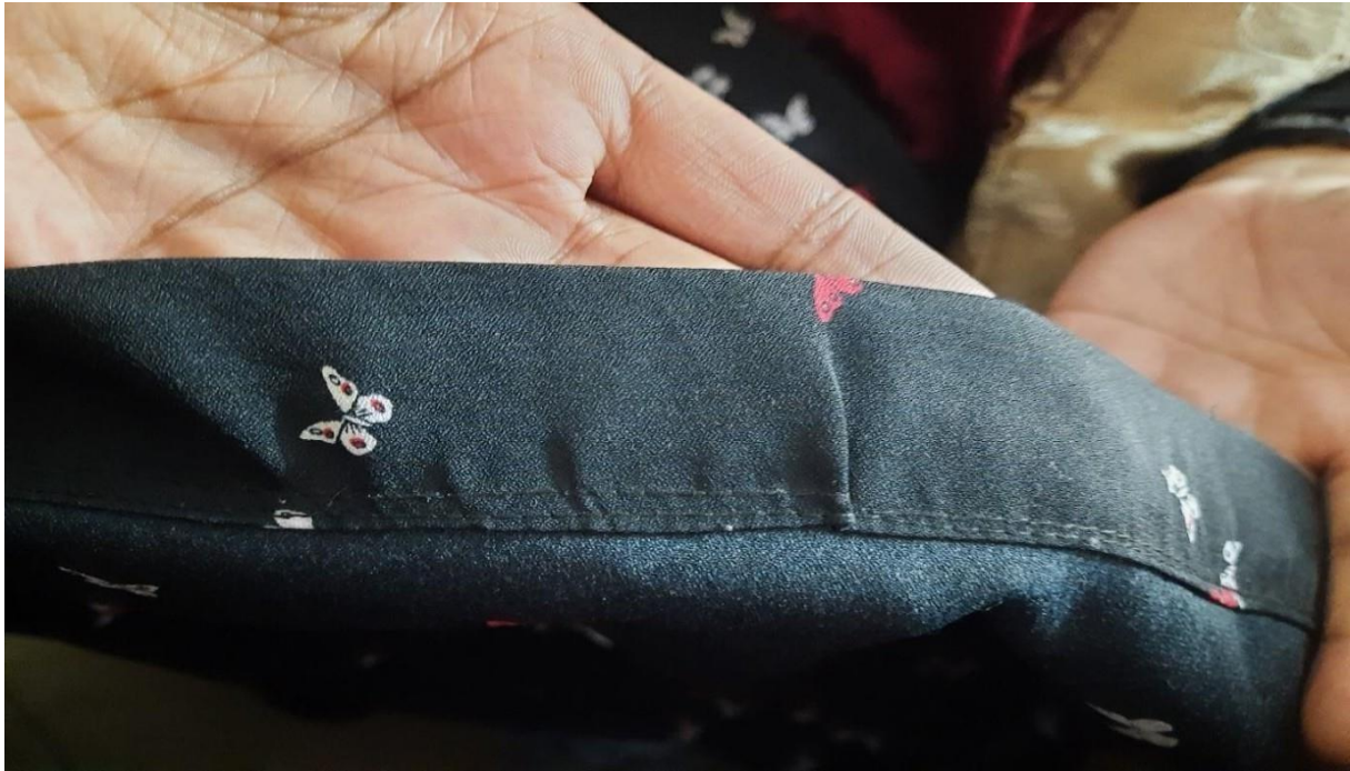
Figure: 2.3.5 Unbalanced Stitch
