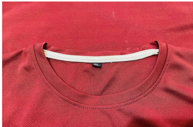
Figure 2.7.2: Main label missing
