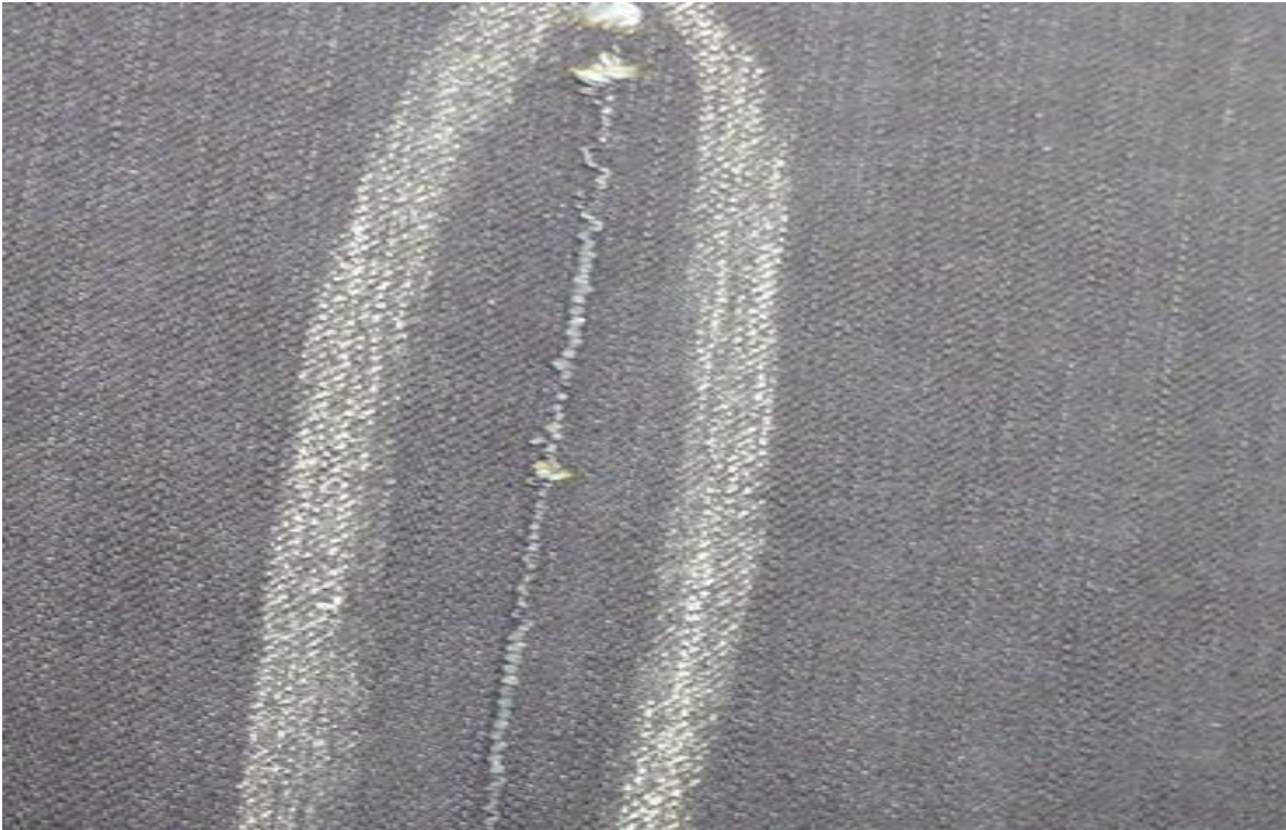
Figure 10: loose warp in fabric.
