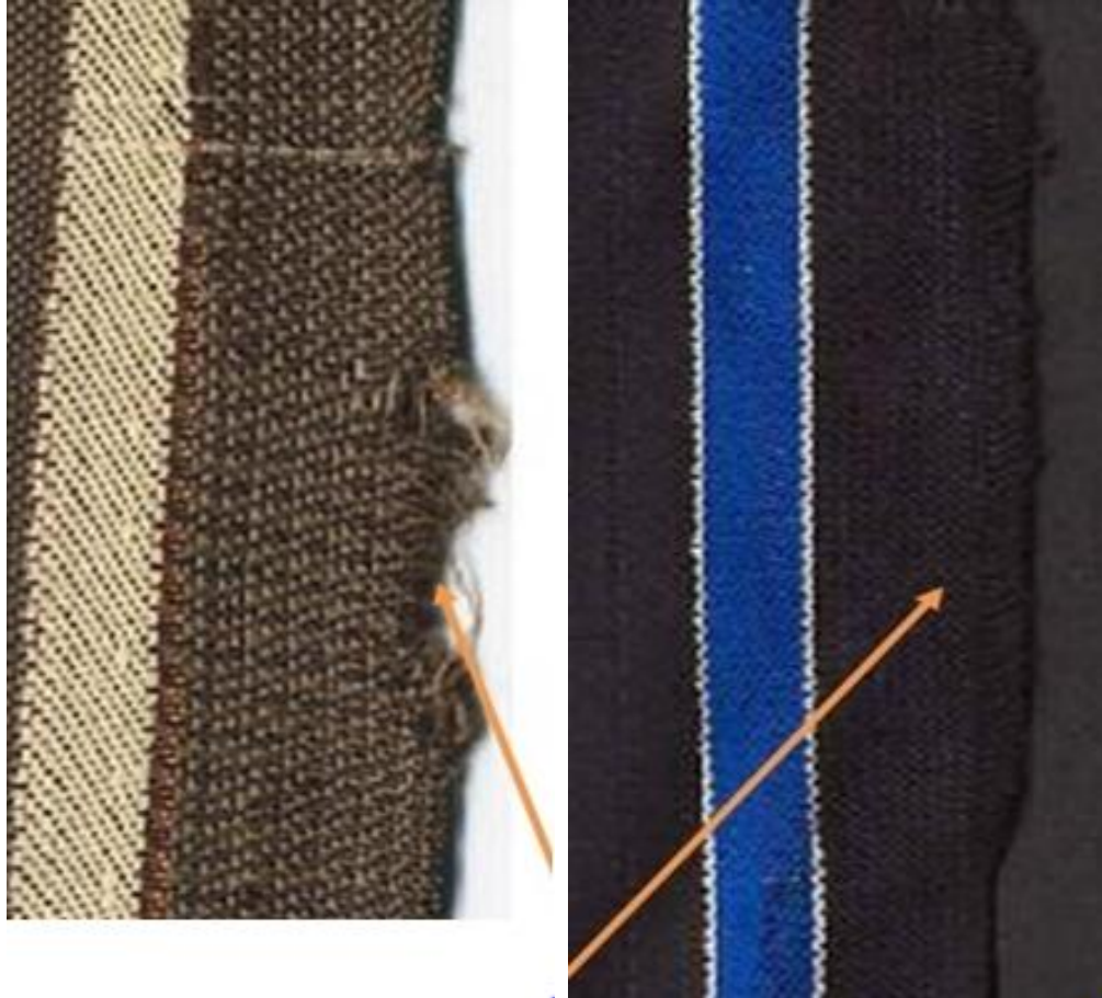
Figure 27: Cut or torn selvedge.
