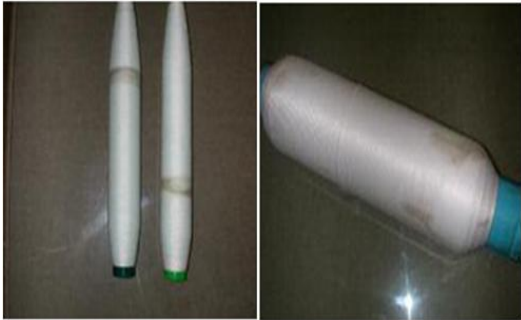
Figure 7: Oil stained yarn.
