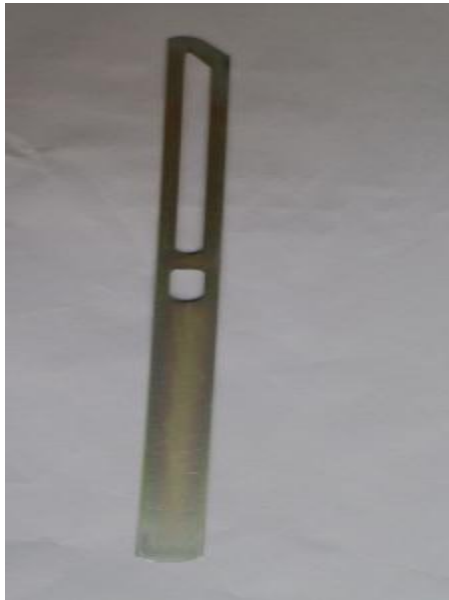
Figure : Drop wire used in Shasha Denims Ltd.
