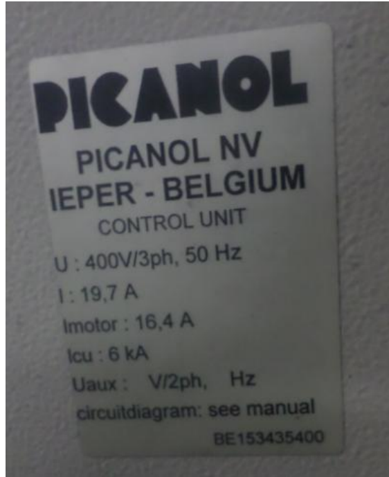
Figure: Specification of picanol omni airjet loom used in Shasha Denims Ltd.
