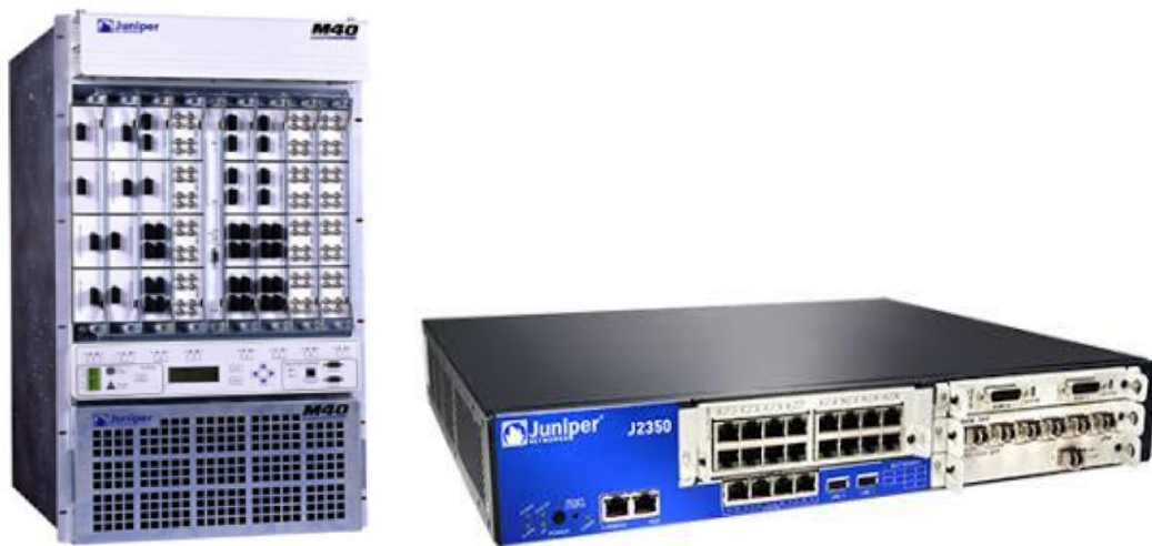
Figure-2.1: Juniper Router [4]
