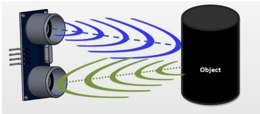
Fig 2.8: Object detecting by Ultrasonic Sensor
