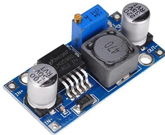
Fig. 3.12 LM2596 Buck Converter
