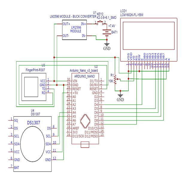
Fig. 4.3 Hardware Connection of Fingerprint attendance system
