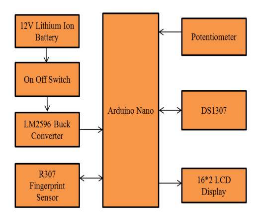
Fig. 4.1 Block Diagram of Based on Fingerprint Student Attending System
