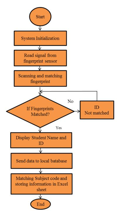
Fig. 4.2 Flow Chart of Based on Fingerprint Student Attending System
