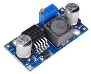
Fig. 3.12 LM2596 Buck Converter
