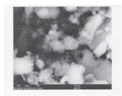
Figure 1: Crystalline structure of eggshell
