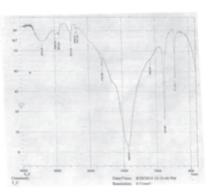
Figure 5: IR Spectrum of eggshell sample (3C)
