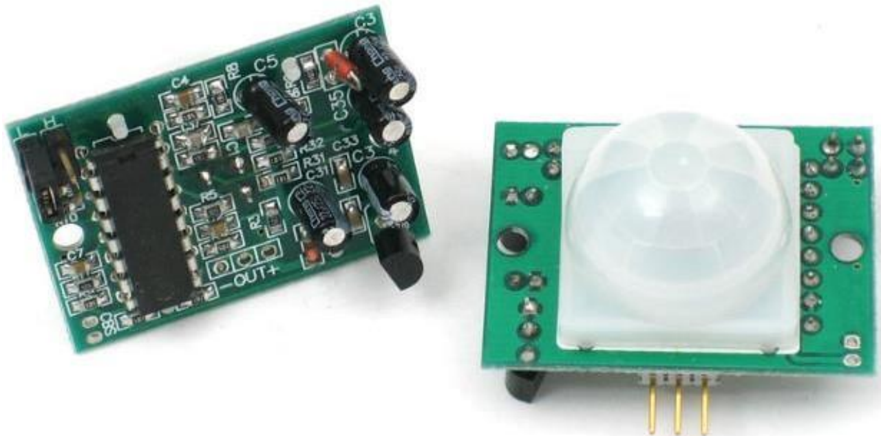
Figure 3.5: PIR motion sensor [ref 11]
