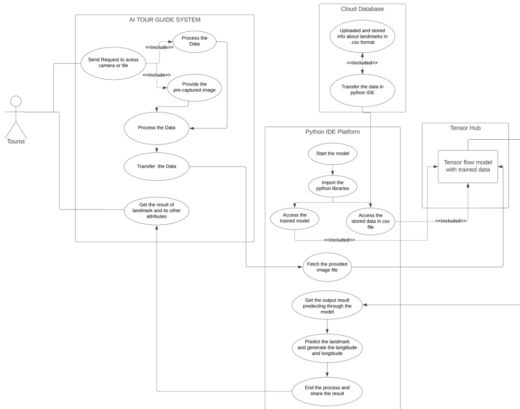
Figure 4: Process of landmark detection through the use case diagram using TensorFlow
