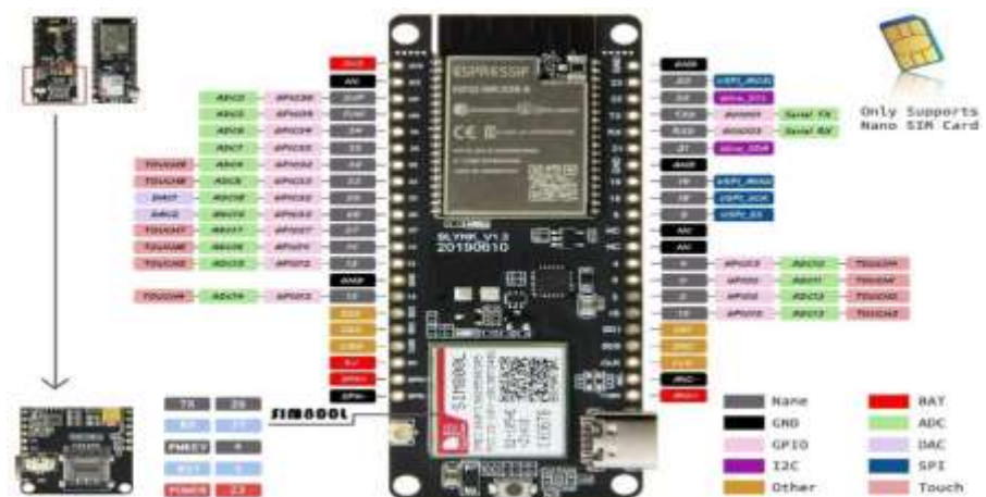
Fig. 3.4: ESP32+SIM800L Pin Out Details.
