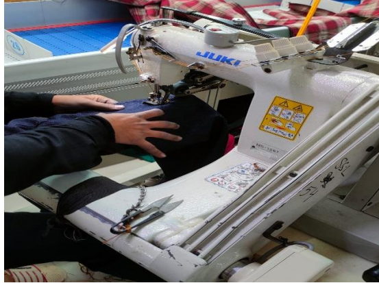
2.2.4 Figure: feed of the Arm chain stitch machine
