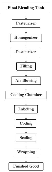
Fig 2.7: Hot fill production flowchart
