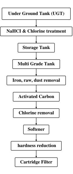
Fig 2.3: Water Treatment Plant flow chart
