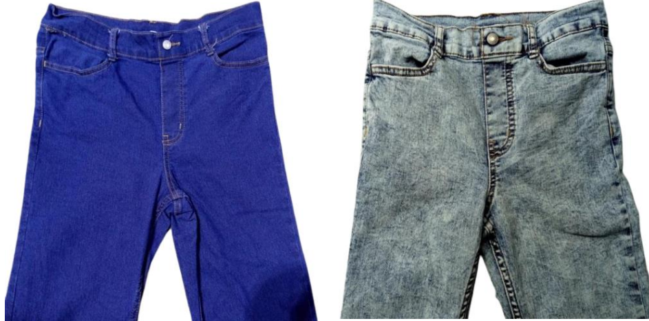
Figure 16: Acid washing effects (with thermocol ball) of before and after acid wash
