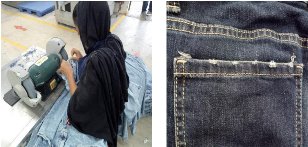
Figure 07: Grinding pocket edges after washing
