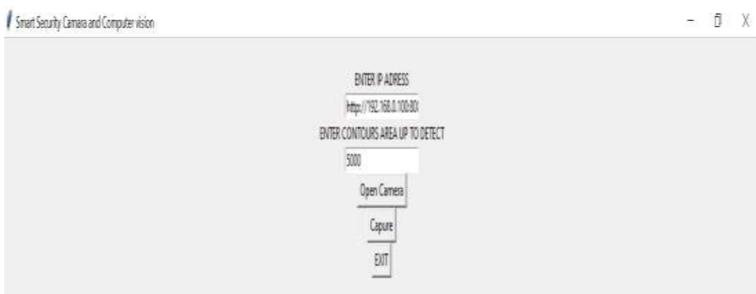
Fig 4.13 IP link http://192.168.0.103:8080/ and contours area selection based on computer vision or video visualization software through the Internet.
