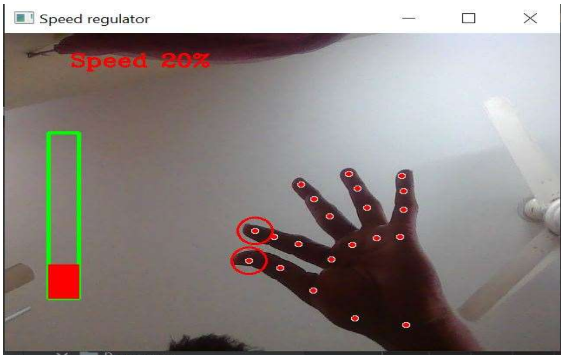
Fig 1.19 Gesture Control Low-Level gap between index and thumb finger
