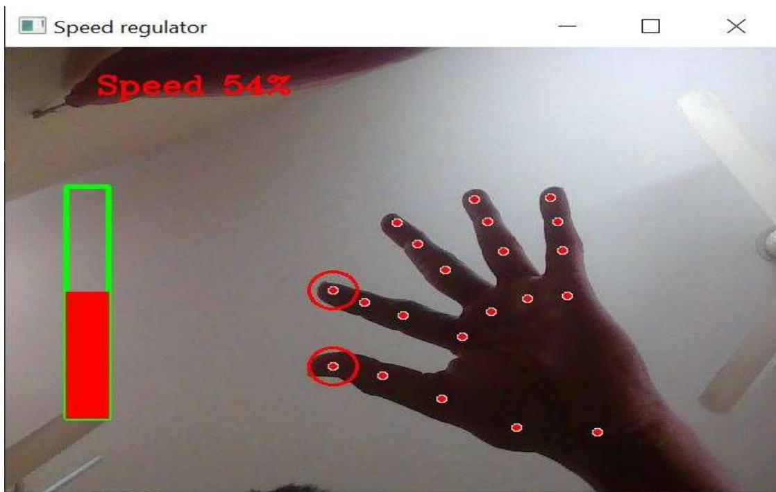
Fig 1.18 Gesture Control Medium Level gap between index and thumb finger.
