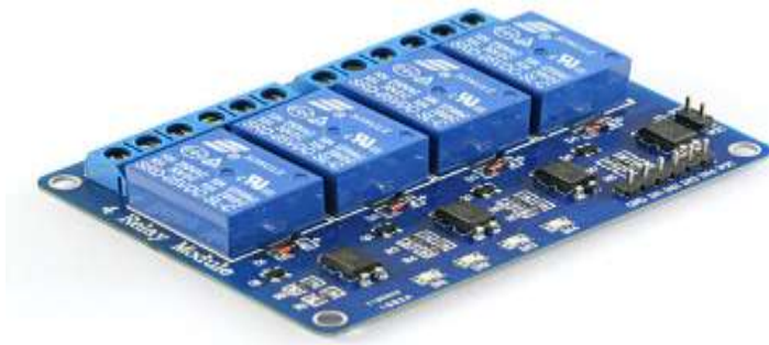
Fig 3.11 5v four channel Relay Module
