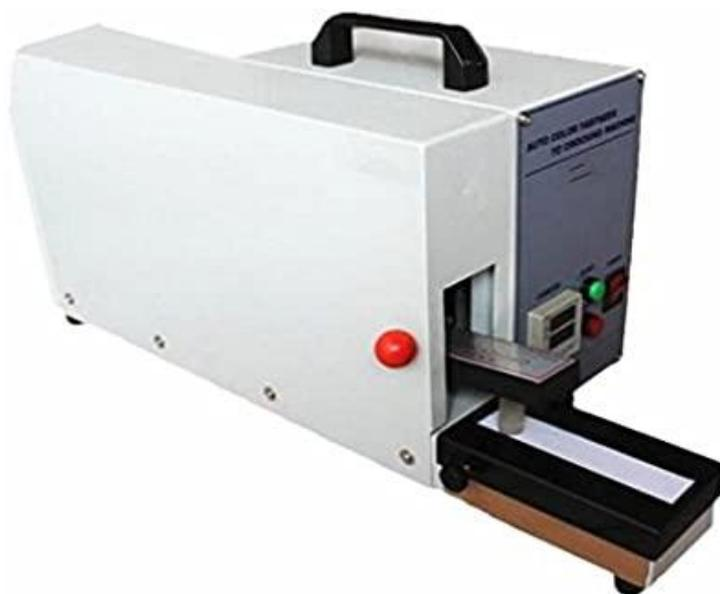
*Figure 3.2.10. Rubbing fastness tester (crock master)*
