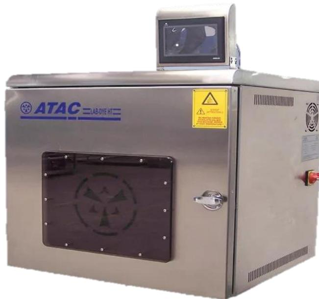
*Figure 1.2.8. ATAC sample dyeing machine*
