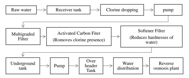
Figure: Process flow chart of Water Treatment Plant
