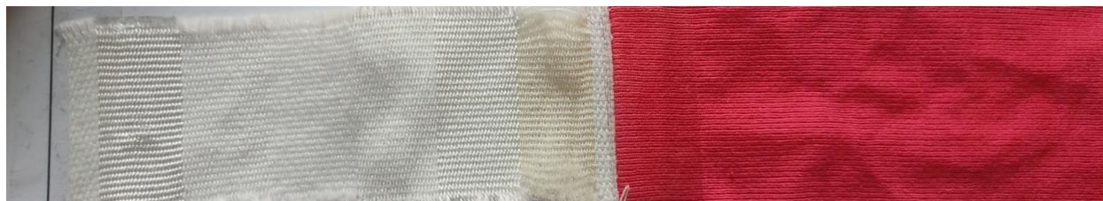
Fig: Color fastness to wash for 1% Red
