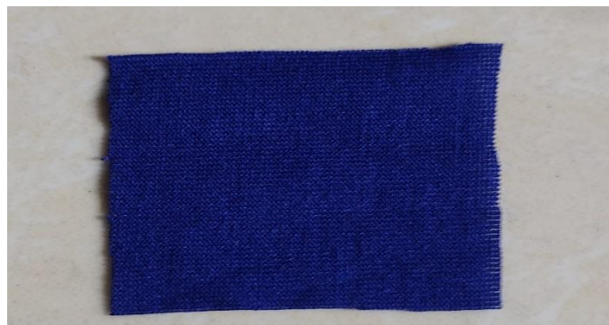
Fig: color fastness to light for 3%( grade: 8)
