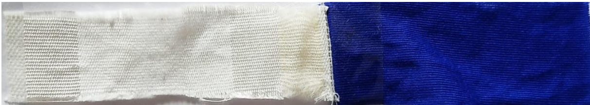
Fig: Color fastness to wash for 2% Blue
