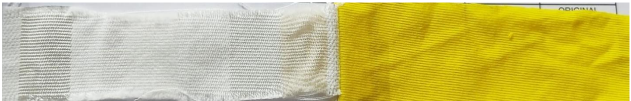
Fig: Color fastness to wash for 3% Yellow
