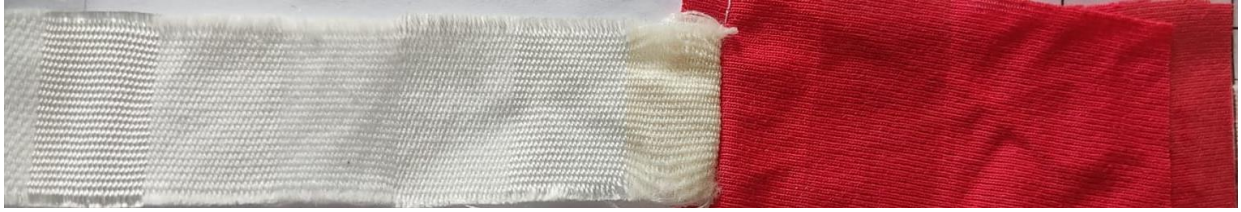
Fig: Color fastness to wash for 3% Red
