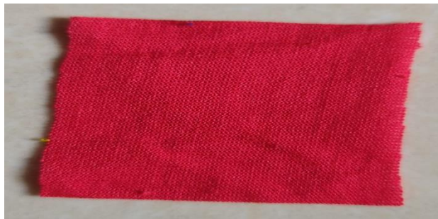
Fig: color fastness to light for 3% ( grade: 7)
