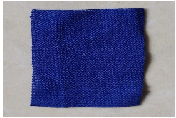
Fig: color fastness to light for 2%( grade: 8)
