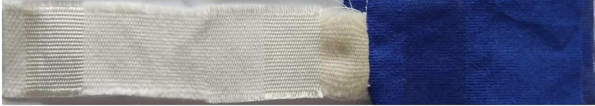
Fig: Color fastness to wash for 1% Blue
