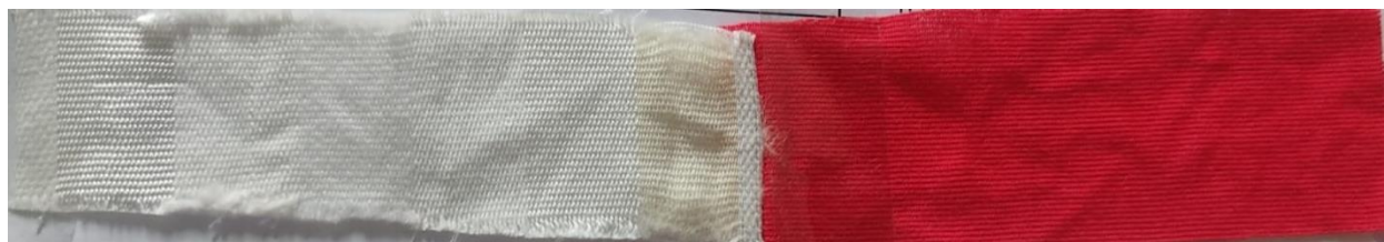
Fig: Color fastness to wash for 1% Red
