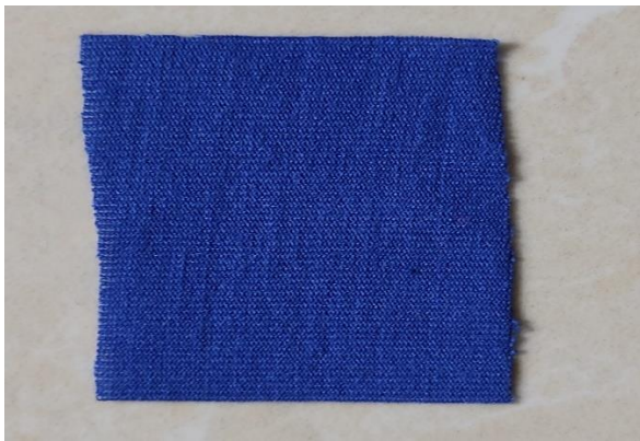
Fig: color fastness to light for 1%( grade: 8)
