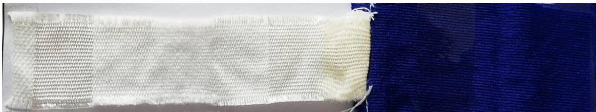
Fig: Color fastness to wash for 3% Blue
