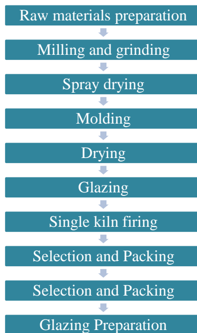
Figure 2. 1: The conventional method of making ceramic tiles involves wet milling, automation, and a single kiln fire.
