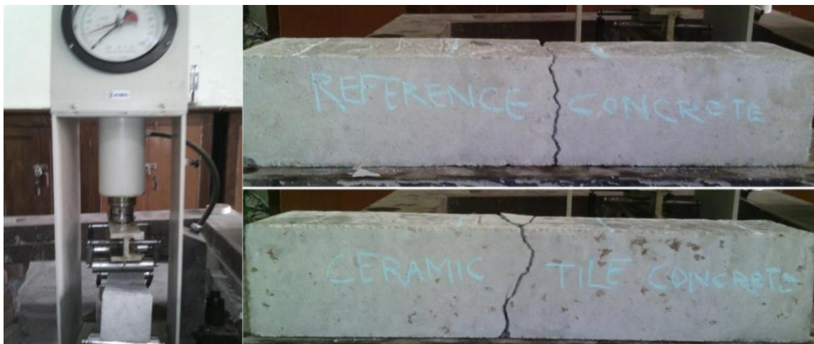
Figure 2. 6: Instrument for measuring flexural strength, with specimen, failed specimen
