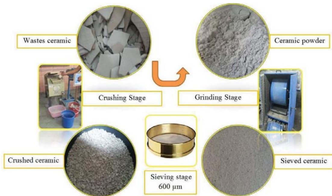
Figure 2. 8: Preparation processes of WCP and CFA.
