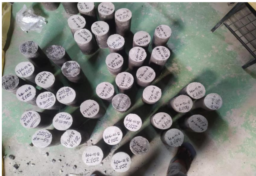
Figure 3. 9: Cylinder are being submerged in the curing pond for curing of 7,14, & 28 days.
