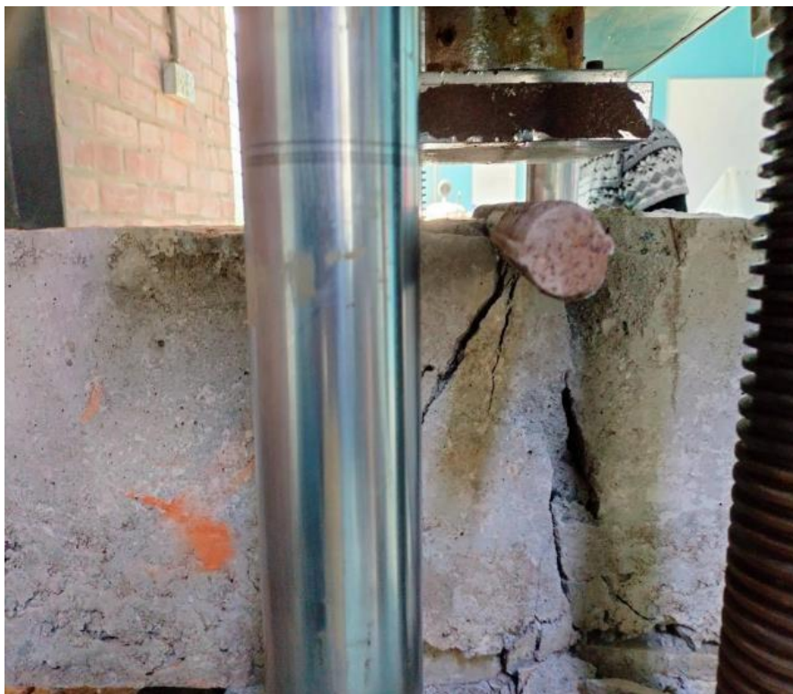
Fig 4.10.2: Beam under flexural strength test at 28 days curing period.
