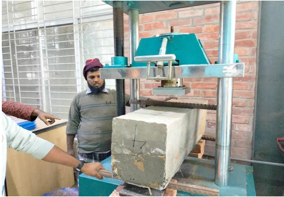
Fig 4.10.1: Beam under flexural strength test at 28 days curing period.
