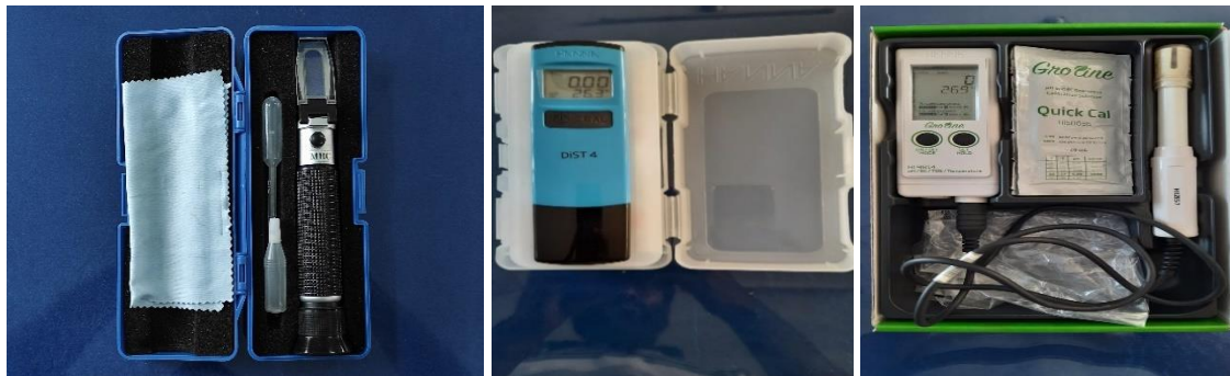
Figure 5: MRC Salinity refractometer, Hanna HI98304 DiST@4 EC-Tester & Hanna HI9814 Multiparameter GroPro pH/EC/TDS/°C (From left)
