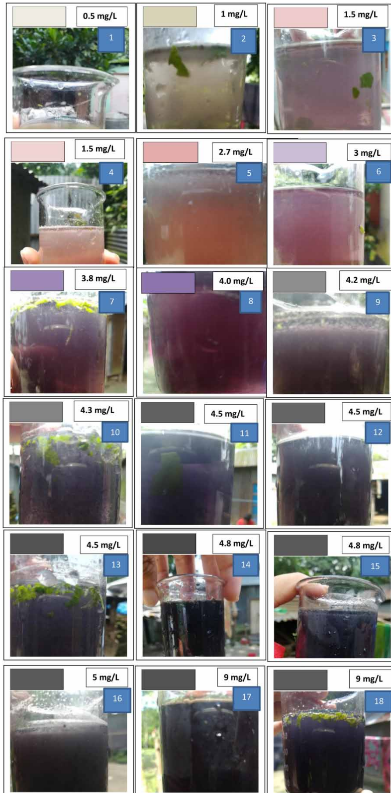
Figure 2 | Guava leaf-induced changes in color groups of the groundwater samples vs. actual iron concentrations of the groundwater samples. Interpretation of the color groups: Whitish: 0.5–1 mg/L; Shades of pink: 1.5–2.7 mg/L; Shades of purple: 3–4 mg/L; Light black: 4.2–4.3 mg/L; Frank black: \geq 4.5 mg/L.
