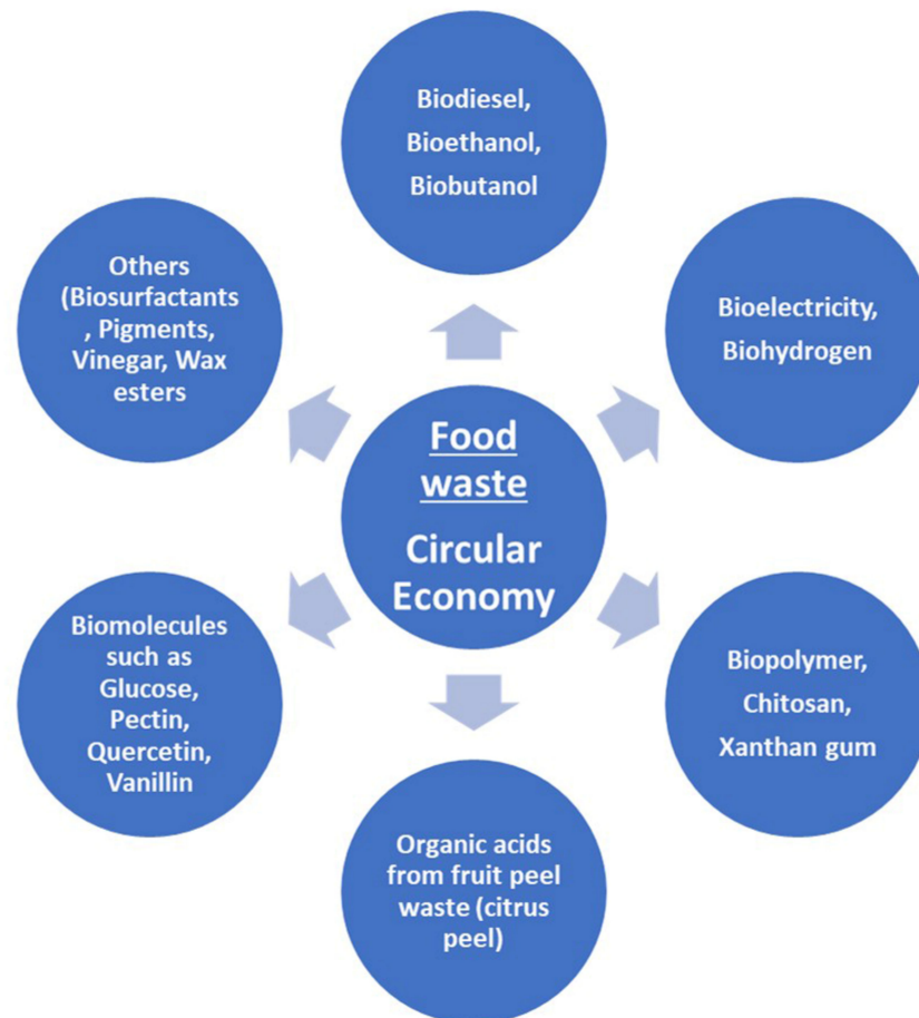
Figure 6. Value-added products and bioenergy are derived from FW through adopting a circular economy.
