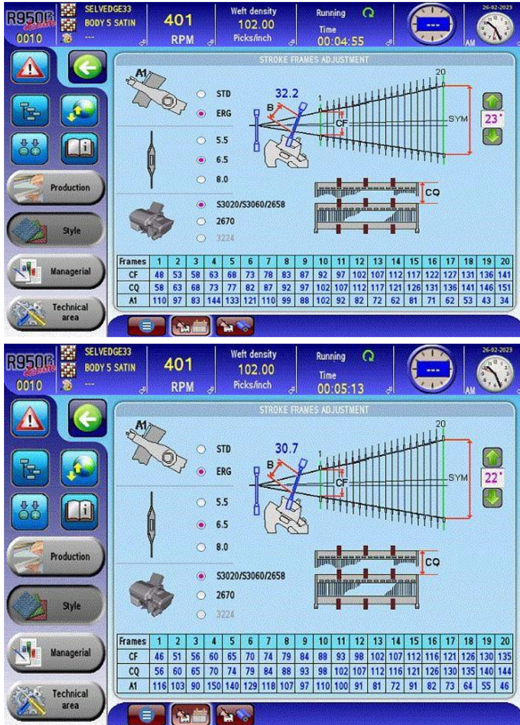
Figure 30: Dobby scale and frame height setting
