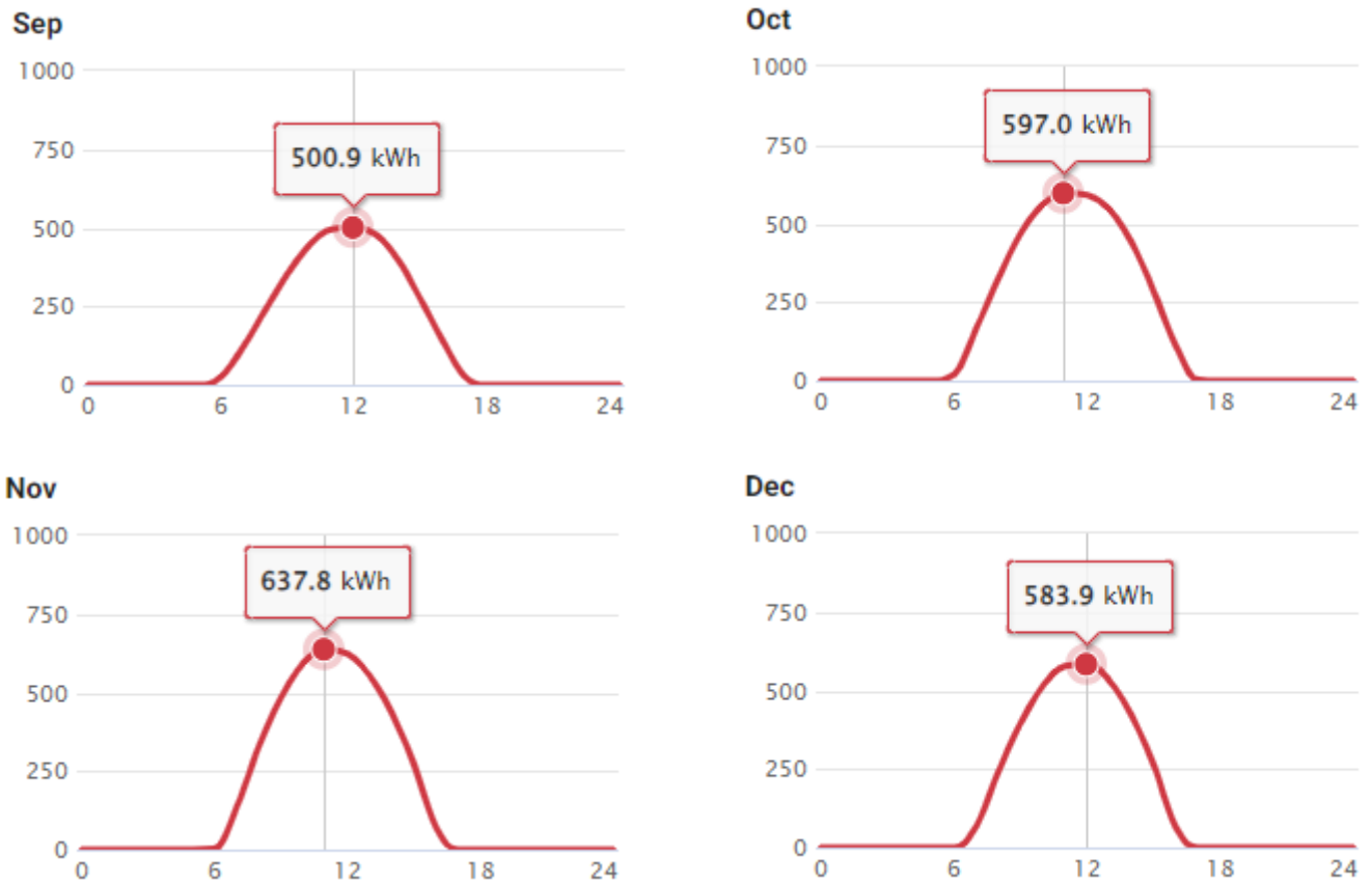
Figure 3.22: Photovoltaic Average Hourly Profiles
