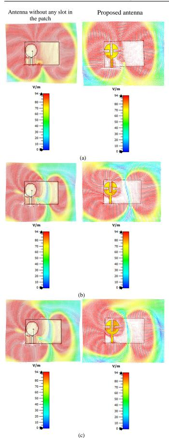
Fig. 6. The surface E-field propagation pattern without any slot in the patch and e proposed antenna at; (a) 1.57 GHz, (b) 2.1 GHz, (c) 2.4 GHz (color online)
