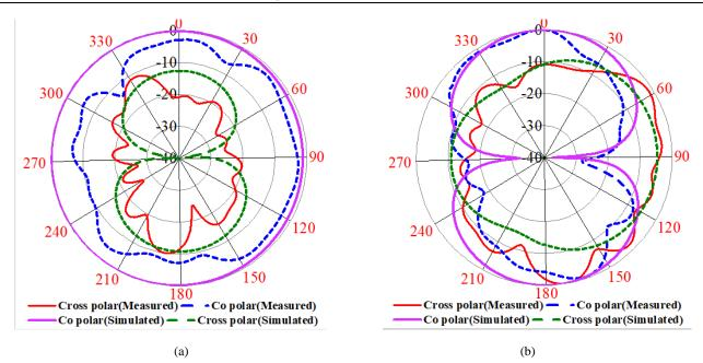
Fig. 9. Laboratory measurement radiation pattern outcomes at 1.57 GHz along; (a) xz-plane (phi=0), (b) yz-plane (phi=90) (color online)
