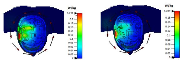
(a) (b) Fig. 14. Simulated Specific Absorption Rate (W/Kg) at; (a) 2.1 GHz, (b) 2.4 GHz (color online)
