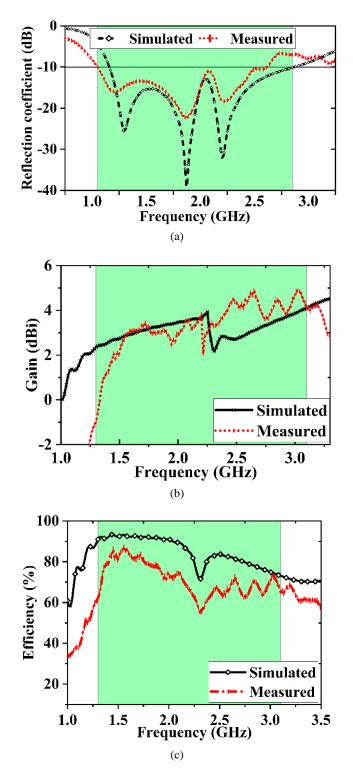
Fig. 8. Laboratory measurement outcomes; (a) Reflection coefficient (S<sub>11</sub>), (b) Peak gain, (c) Radiation efficiency (color online)
