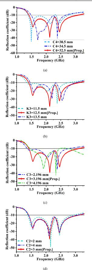
Fig. 3. The influences of changing various parameters on the proposed SEPDGA; (a) C4 parameter, (b) K3 parameter, (c) C3 parameter, (d) C2 parameter (color online)
