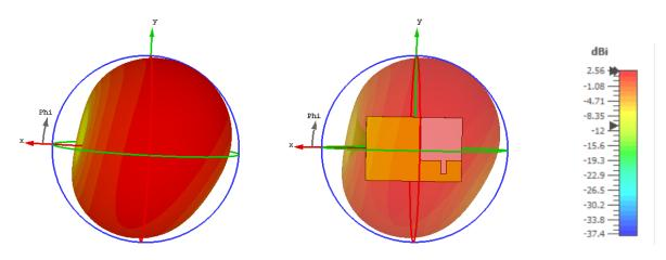
Fig. 10. 3-dimensional radiation pattern view at 1.57 GHz; (a) non-transparent view, (b) transparent view (color online)
