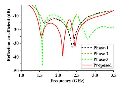
Fig. 2. Simulated reflection coefficient for each step of the evolution phase (color online)
