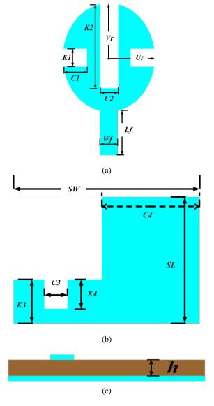
Fig. 4. Optimum layout of the proposed SEPDGA antenna; (a) Patch radiator, (b) Back radiator, (c) Side-view (color online)
