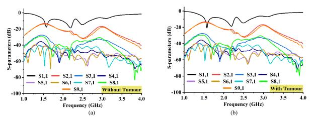
Fig. 13. Simulated scattering parameters; (a) with healthy head, (b) with tumor-bearing head (color online)
