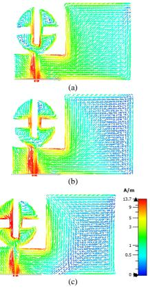
*Fig. 5. Surface Current density at resonance point;* (a) 1.57 GHz, (b) 2.1 GHz, (c) 2.4 GHz (color online)
