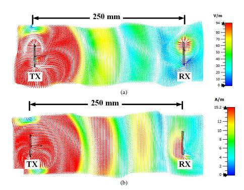
Fig. 11. Field response between transmitter and receiver; (a) E-field and (b) H-field (color online)
