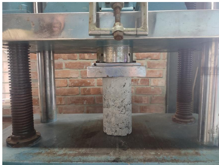
Figure 3.6.1: Compressive Strength Test
