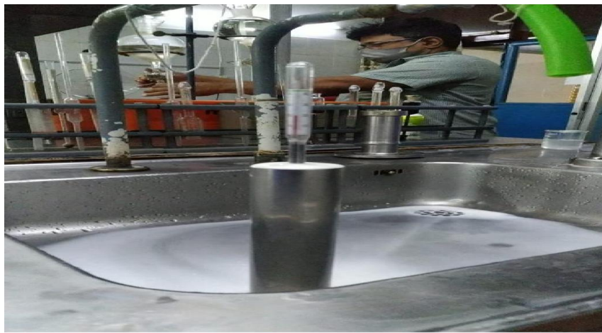
Figure 5.4 :- CLR/Density Measurement Test
