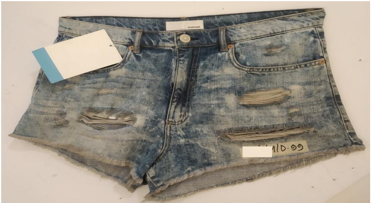
Fig: Acid, Destroy, Grinding, Fraying
