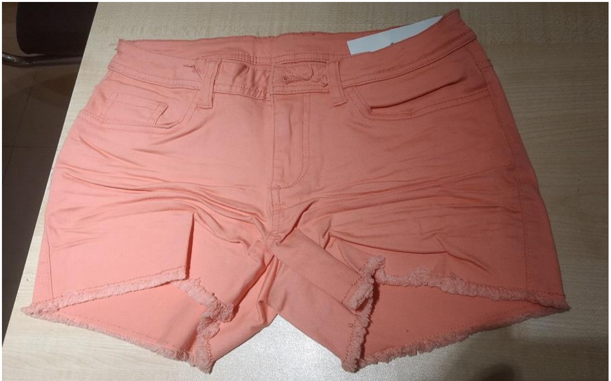
Fig: Over Dyed, 3D (Crinkle), Fraying
