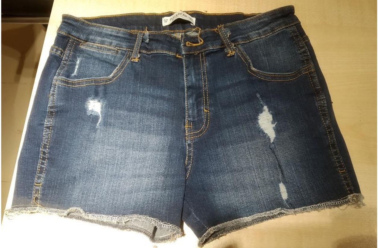
Fig: Bleach, Destroy & Grinding
