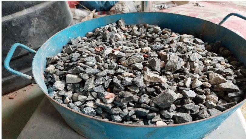
**Figure 3.3.2:** Coarse Aggregate
