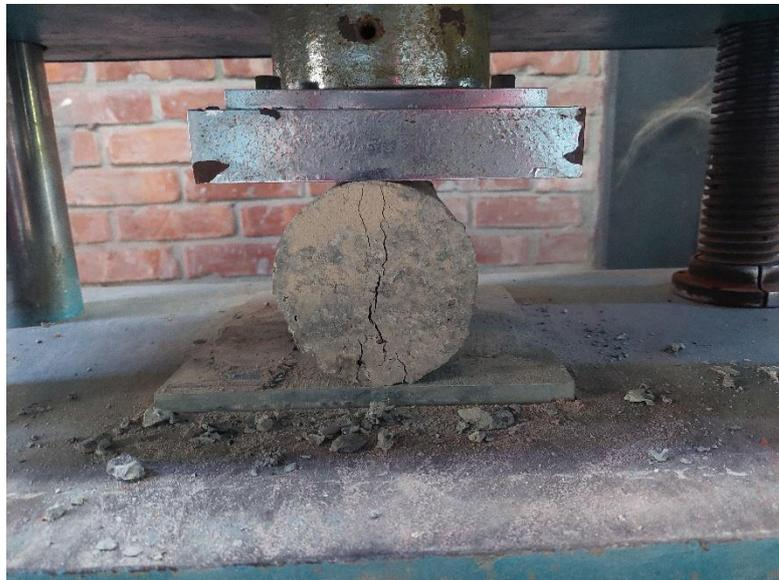
**Figure 3.6:** Split Tensile Test
