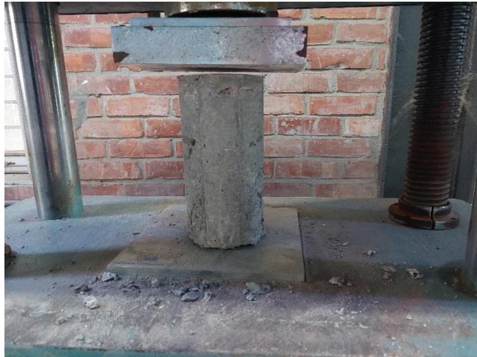
**Figure 3.5:** Compressive Strength Test
