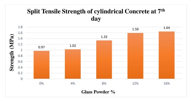
**Figure 4.4.1:** Split Tensile Strength of Cylindrical with respect to % of Glass Powder at 7<sup>th</sup> day.
