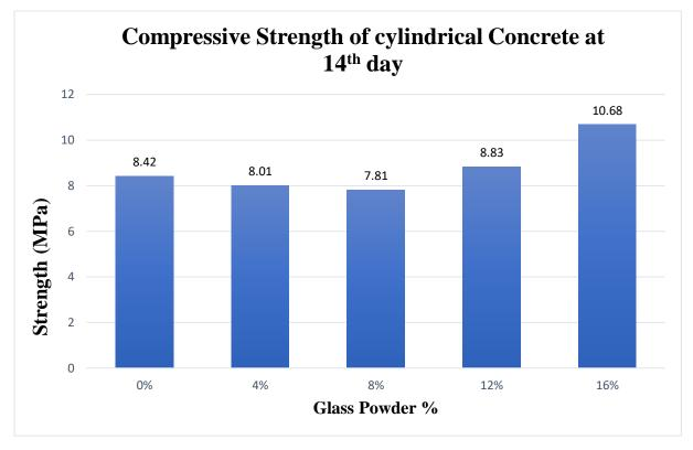
Figure 4.3.2: Compressive Strength of Cylindrical with respect to % of Glass Powder at 14<sup>th</sup> day.
