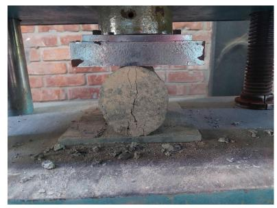
Figure 3.6: Split Tensile Test
