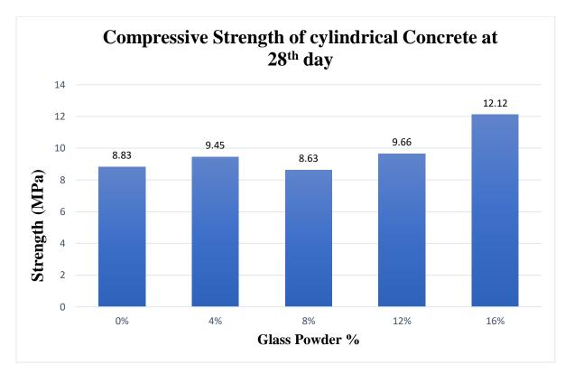
Figure 4.3.3: Compressive Strength of Cylindrical with respect to % of Glass Powder at 28<sup>th</sup> day.
