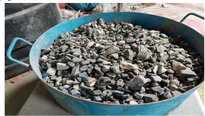
Figure 3.3.2: Coarse Aggregate
