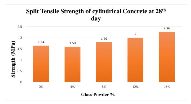
Figure 4.4.3: Split Tensile Strength of Cylindrical with respect to % of Glass Powder at  $28^{\text{th}}$  day.
