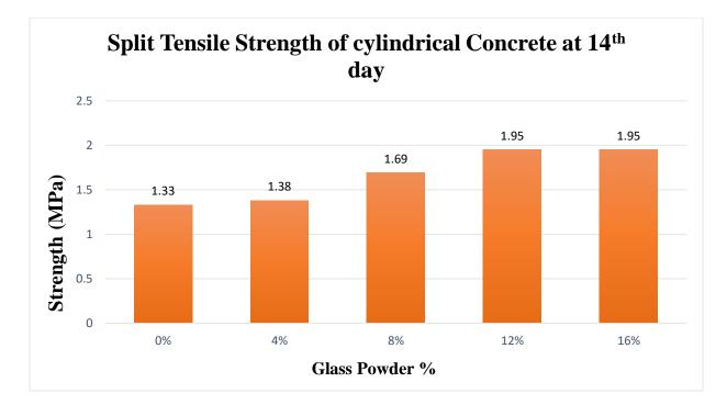
Figure 4.4.2: Split Tensile Strength of Cylindrical with respect to % of Glass Powder at  $14^{th}$  day.
