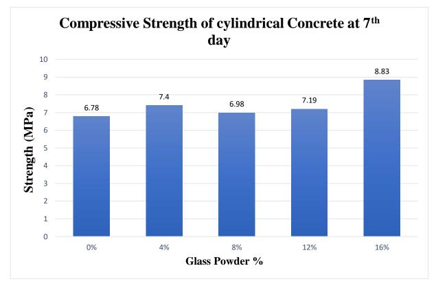
Figure 4.3.1: Compressive Strength of Cylindrical with respect to % of Glass Powder at 7<sup>th</sup> day.
