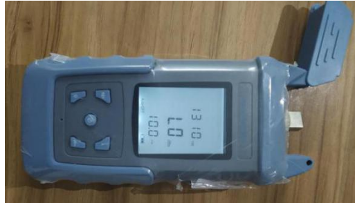
Image 3.19 : Optical Power Meter
