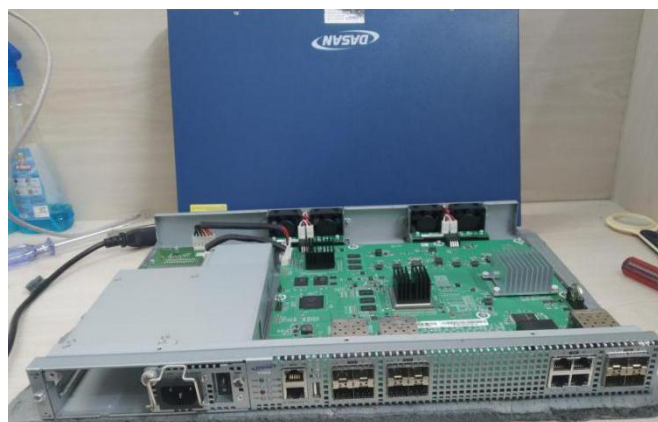
Image 3.5 : Dasan 8port GPON OLT
