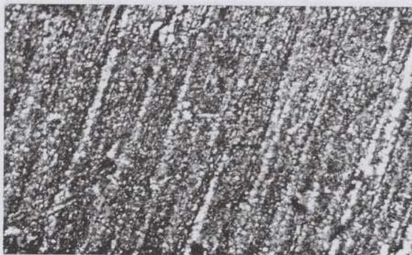
Plate 1d) Microstructure of sample heat treated at 350 °C and holding time of 4 hrs at 93 % deformation
