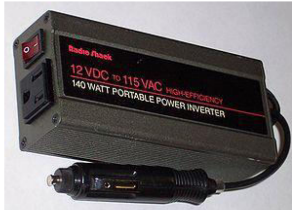
Fig. 3.12: Inverter designed to provide 115 VAC from the 12 VDC source provided in an automobile.
