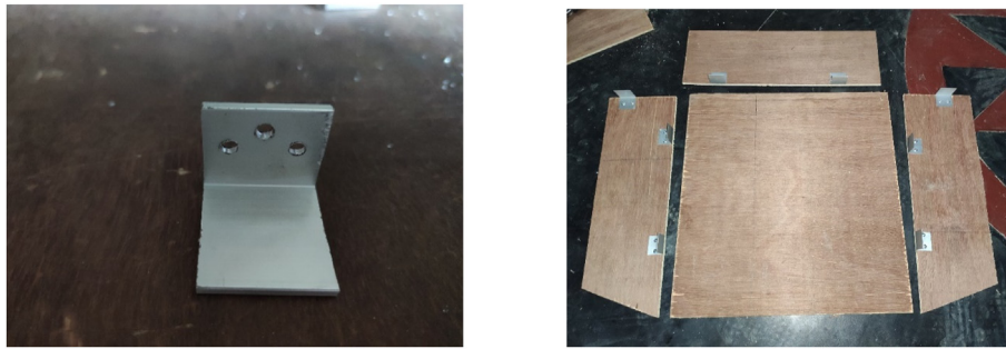
Figure 2. Aluminum joint clamp and well-shaped plywood box.
