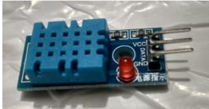
Fig. 3: DHT11 sensor (Own captured).
