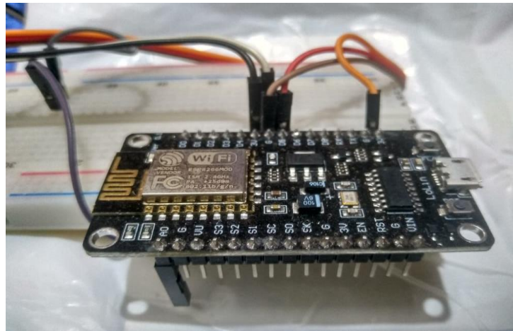
Fig. 2: ESP8266 NodeMCU (Own captured).
