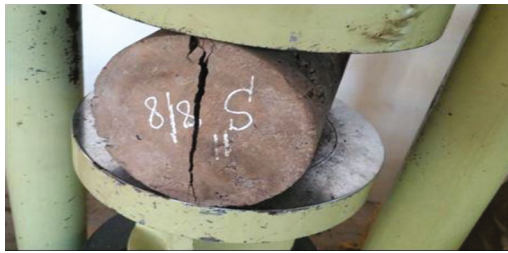
FIGURE 7: The split tensile test specimen.
