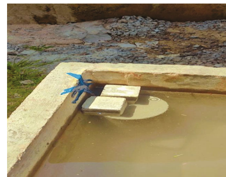
FIGURE 6: Specimens kept under curing for 28 days.
