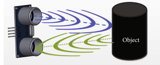
FIGURE 4: Ultrasonic wave travel in air.
