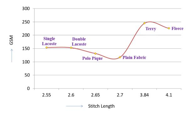
From this chart we can see various types of single jersey knit fabric GSM and stitch length comparison. Where the different stitch length shows different GSM results.
