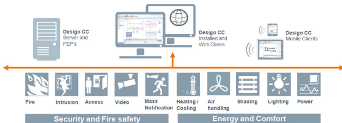
Fig. 11 Shows Building automation and management systems. Source Siemens Switzerland Ltd, 2016
