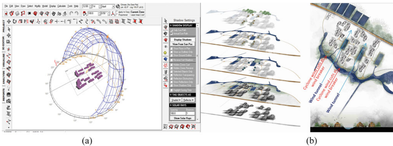
Fig. 5 a Autodesk Ecotect analysis for shadow b Using the shadow analysis for cluster planning
