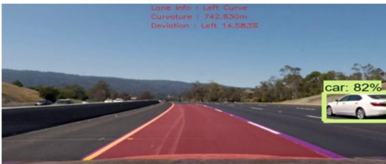
Fig. 5 Lane projection and object detection viewed on frame
