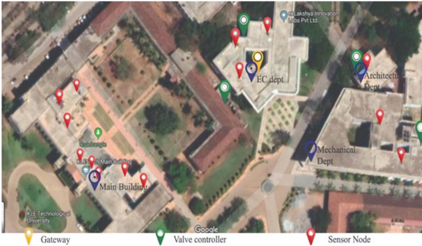
Fig. 4 Gateway and sensor node deployed on campus
