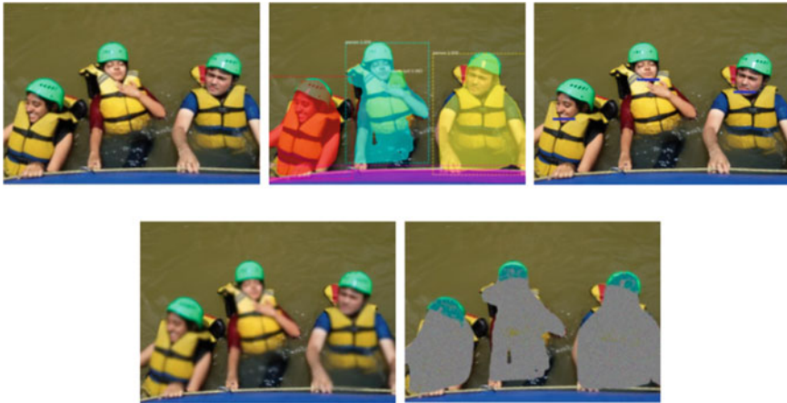
Fig. 5 First image is the input on which we have generated the following outputs. The second image shows the bounding boxes and segmented instances. The faces of the people that can be seen in the picture are detected and recognized in the next image. The bottom-left image is the output of the blurring algorithm, and the last image is the output of the encryption algorithm
