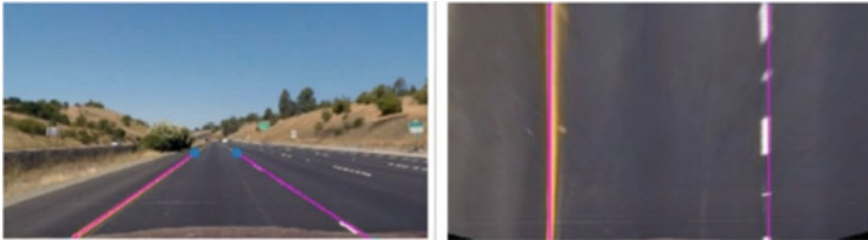
Fig. 3 Perspective transform from vehicle to sky view
