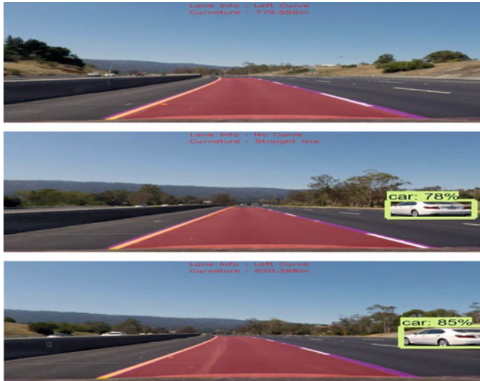
Fig. 8 Result showing lane detection, object detection, and curvature information
