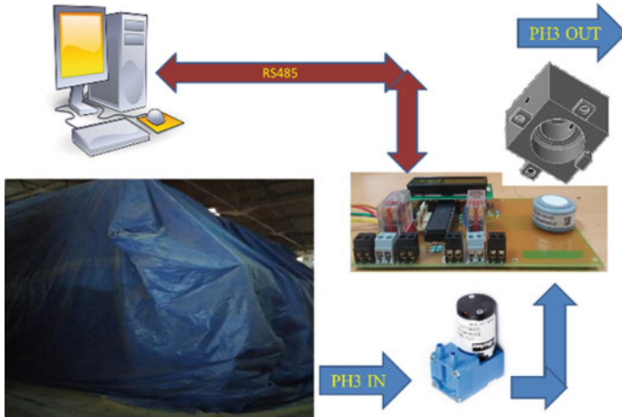
Fig. 5 Schematic view of working principle of FUMON
