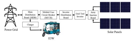
Figure 11. Net metering based electric three-wheeler charging station.
