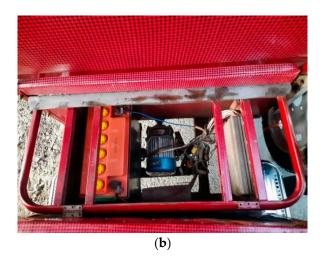
Figure 2. Lead acid battery pack location in E3W under (a) the passenger seat and (b) the driver seat.
