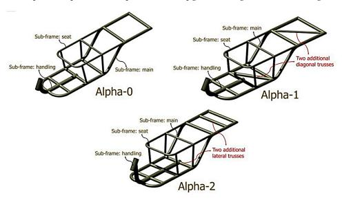
**Figure 8.** Alpha frames for E3W [27].
