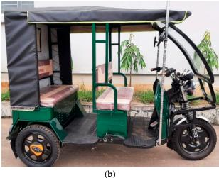
Figure 1. Electric three-wheelers: (a) Easy Bike (b) Mishuk.
