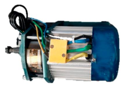
Figure 4. A brushless DC motor used in E3Ws.
