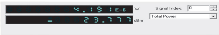
Figure 11: The signal at the receiver side in the presence of the operating signal wavelength of 850 nm and divergence of a beam of 0.25 mrad.
