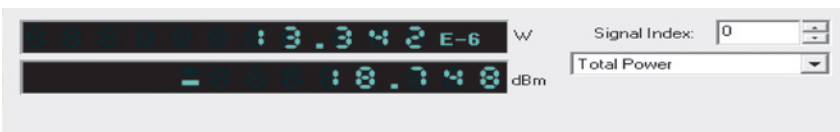
Figure 13: The signal at the receiver side in the presence of the operating signal wavelength of 1550 nm and divergence of a beam of 0.25 mrad.
