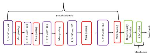
Figure 4. Modified VGG19 architecture.
