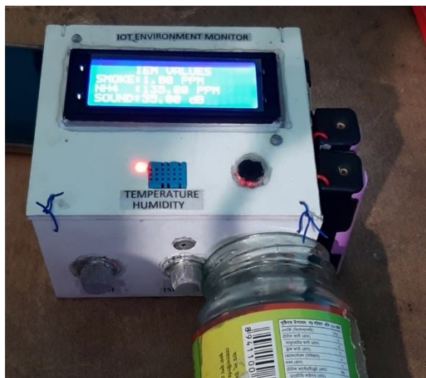
Fig. 6. Experimental results of detecting and/or measuring smoke, NH 4 , and fire.
