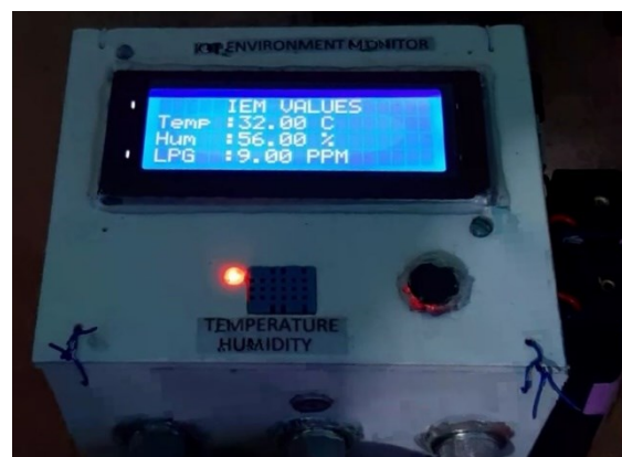
Fig. 5. Experimental results of temperature, humidity, and LPG gas.
