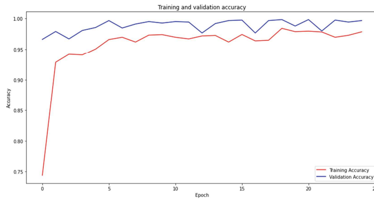
Fig. 4. Accuracy plot for VGG16 transfer learning model’s training and validation
