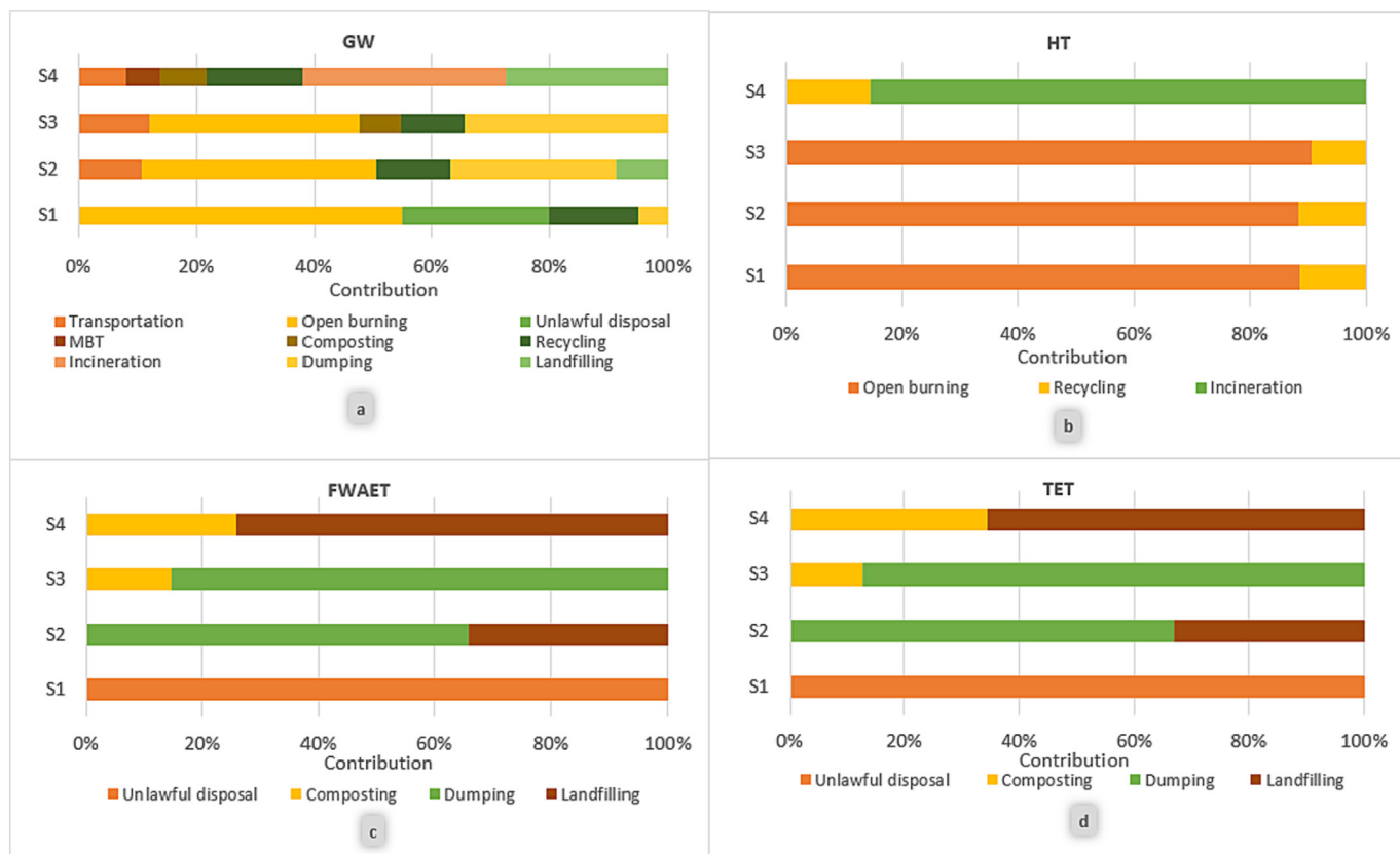
Fig. 8. Impact potential of HCWM (a, b, c & d showing effects of GW, HT, FWAET & TET respectively for four scenarios, S1 to S4) (Alam and Mosharraf, 2020).
