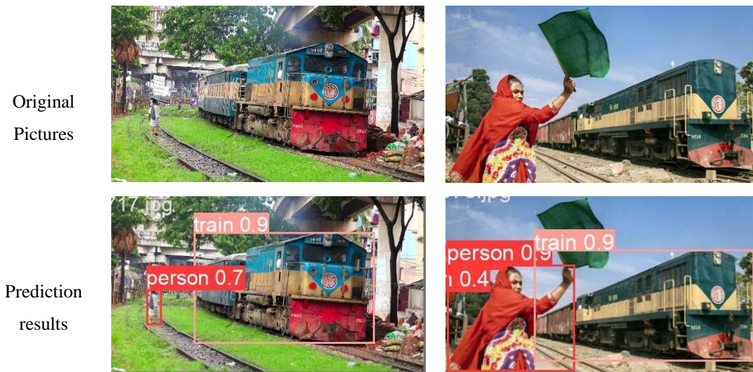
Figure 4.2.4: Output of YOLOv5x
