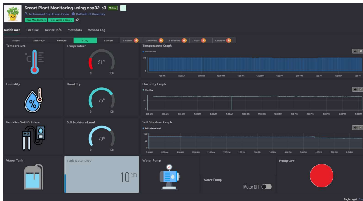
fig 5.2: Blynk interface for plant monitoring
